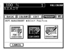
2 If you want to reset all the counters of registered departments, press the ALL key and then the SET key. If you want to reset the counter of a specific department, key in the access code (5 digits) of that department with the digital keys, then press the SET key.
